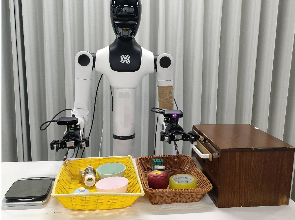
Figure 8: Real-world experimental setup and task suite. The TienKung 2.0 dual-arm robot executing diverse manipulation tasks. The suite comprehensively evaluates both synchronous bimanual coordination and high-precision single-arm motor control.
